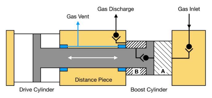
Diagram 1: Booster cylinder operation diagram
