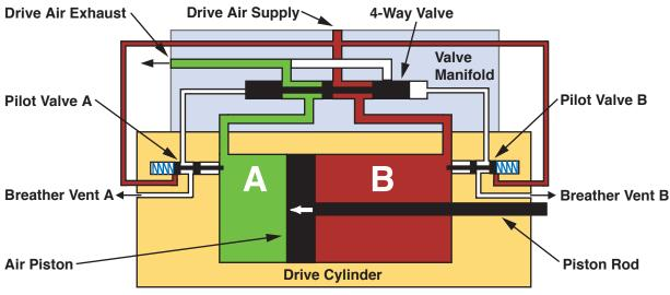
Diagram 2: Drive section operational diagram
