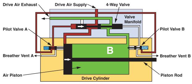
Diagram 3: Drive section operational diagram
