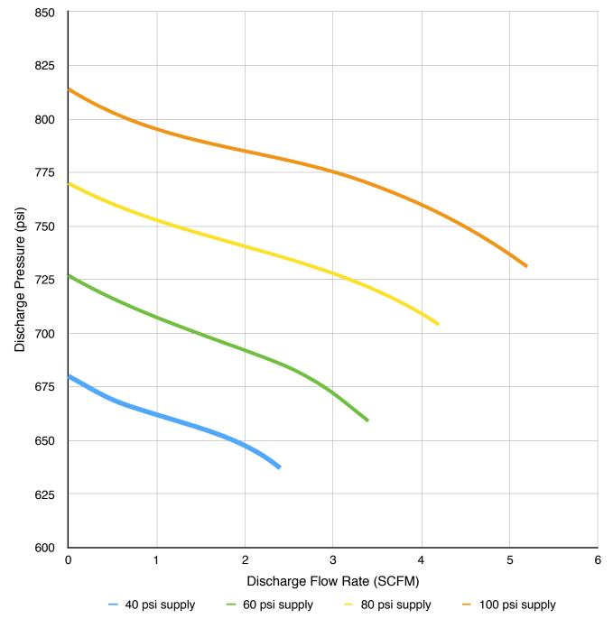
420TAAV090 - Discharge Pressure VS Flow Rate Drive Pressure 80 psi & Gas Supply Pressure Varies
