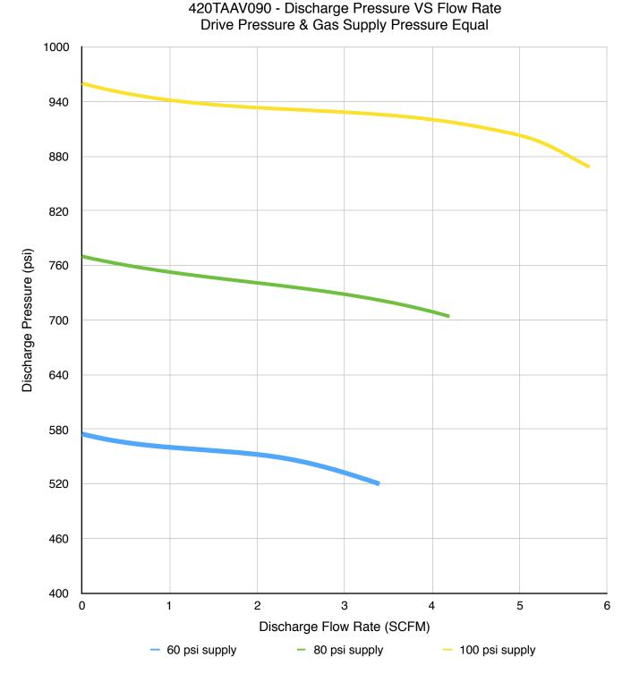
Midwest Pressure Systems, Inc. • 850 Transport Drive • Valparaiso, IN 46383 • USA Phone 219-462-0070 • Fax 219-318-2277 • Web Site <u>www.midwestpressuresystems.com</u> The graph below shows a performance curve of the 420TAAV090 gas pressure booster. In the graph, the drive pressure is held constant at 80 psi and gas supply pressures vary as shown below. Use this curve to size the 420TAAV090 gas pressure booster for a given application.
